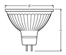
P MR16 DIM 3.4 W/827 GU5.3, P MR16 DIM 3.4 W/830 GU5.3, P MR16 DIM 3.4 W/840 GU5.3, P MR16 DIM 5 W/827 GU5.3, P MR16 DIM 5 W/840 GU5.3 P MR16 35 36° DIM 5 W/827 GU5.3, P MR16 35 36° DIM 5 W/840 GU5.3
